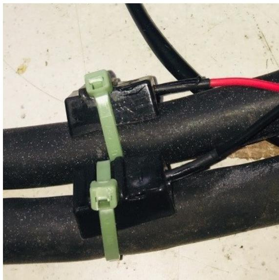
**Figure 12b. Zip Tie the IDC and the Charger DC Cable together**
